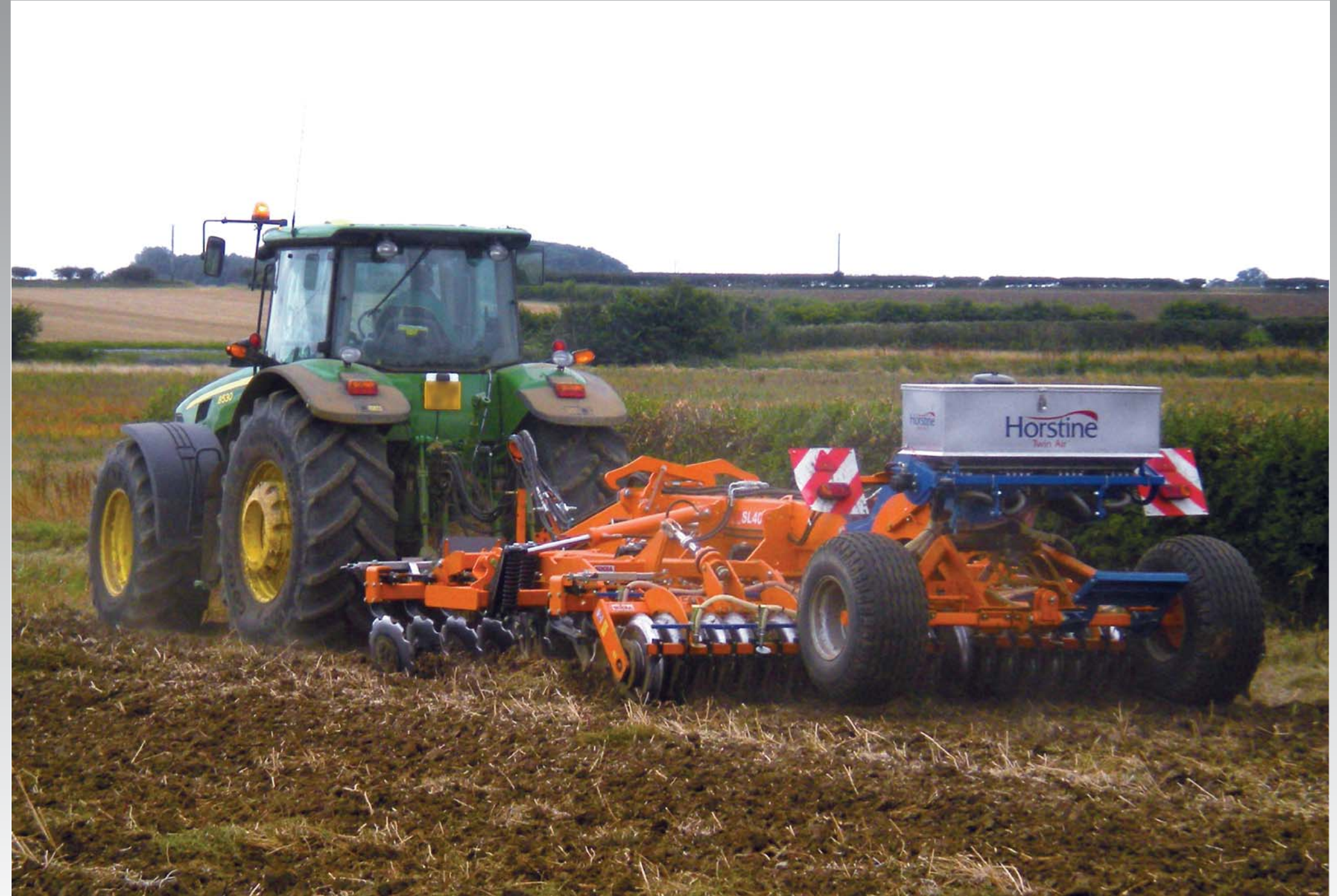
Horstine Twin Air fitted to Simba SL 400 cultivator (Lincolnshire)
