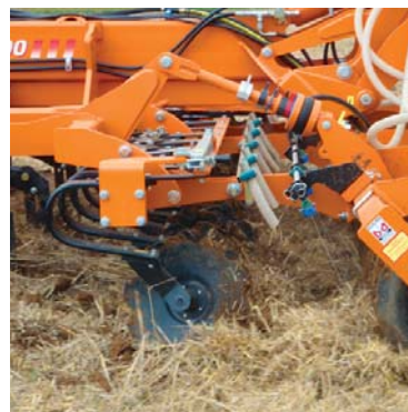
Band application nozzle is unaffected in windy conditions
